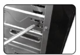
Fasten with screws or tool-free lock.
