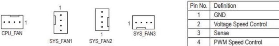
For headers such as these, there is usually an option within BIOS/UEFI to set the control mode to either PWM or DC. First, connect the hub to the fan header. Enter BIOS/UEFI mode and set the control mode for the connected fan header to PWM mode. Some illustrations below:
