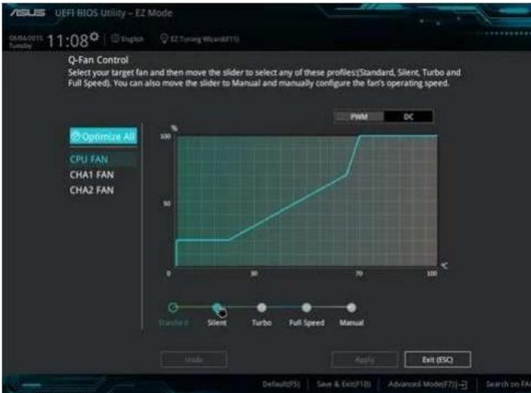
To Test if your PWM is functional: Go to Speed Settings on your BIOS/UEFI for the connected fan header. Toggle the speed between full speed and silent mode to ensure that PWM functions are working.
