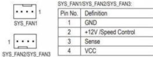
We can see that *Pin No. 4* uses *VCC* and *Pin No. 2* has *+12V/Speed Control*. As a result this header does NOT support PWM, and as a result will NOT work with AeroCool hub.
